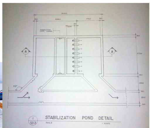
Design of Stabilization Pond at Dipolog Boulevard
